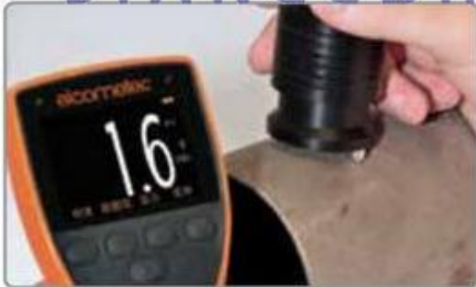
整体式分体式探头测得的粗糙度高达500µm (20mils)
